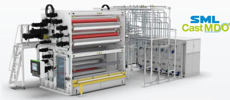
Cast MDO technology marks a significant development in mono-oriented PE film production. By combining precise thickness control across a broad thickness range, outstanding optical properties, and customisable barrier options, it provides packaging manufacturers with a versatile and sustainable solution that meets the highest standards of quality, efficiency, and performance.
