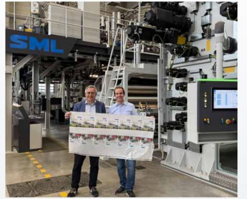
SML's latest cast film lines with an integrated MDO unit are designed to manufacture a wide range of MDO-PE films with different thicknesses and excellent barrier functionalities. These monomaterial films are characterised by their high transparency and very good mechanical properties. Further processing on conventional machinery is straightforward and was tested satisfactorily.
