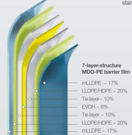
The resulting 17 µm MDO-PE barrier film has the following barrier properties given a
