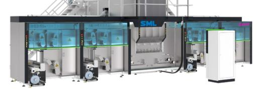
colour changes contribute significantly to the overall production efficiency. With output quantities of up to 160 kg for PP and of up to 110 kg for PA6, SML's Austrofil<sup>®</sup> HT spinning lines guarantee maximum efficiency with smaller batches.
