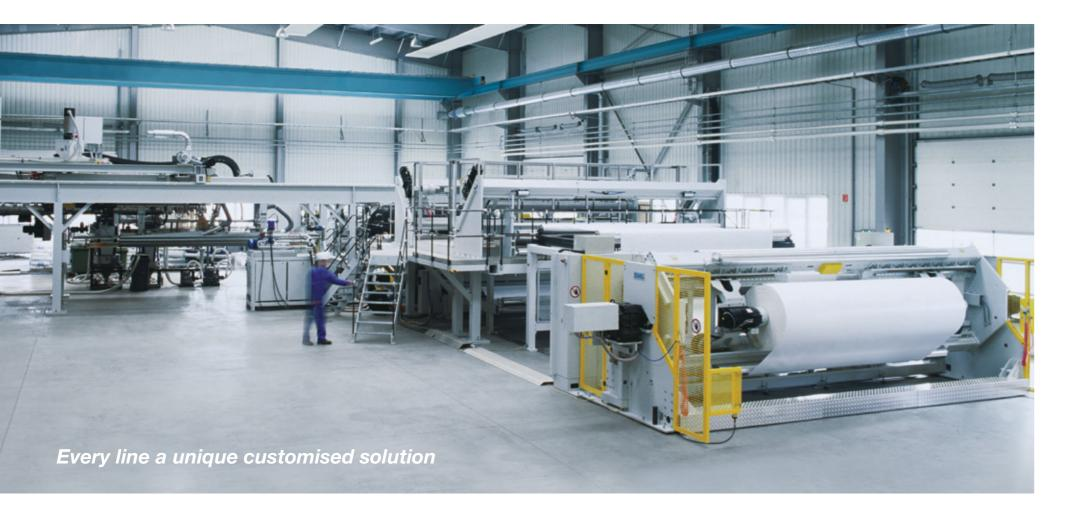
The coating of wide products has been one of the core competencies of SML for decades. One characteristic all these lines have in common is a **very massive machine frame** to withstand the high web tensions and **to avoid vibrations**.
