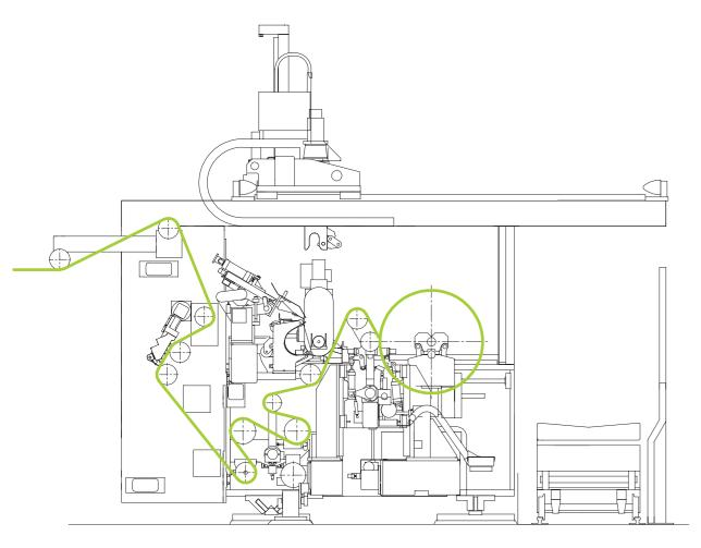
The inline-slitting process can be carried out either with bleed trims or without bleed trims in combination with banana rolls for the separation of the single webs.
