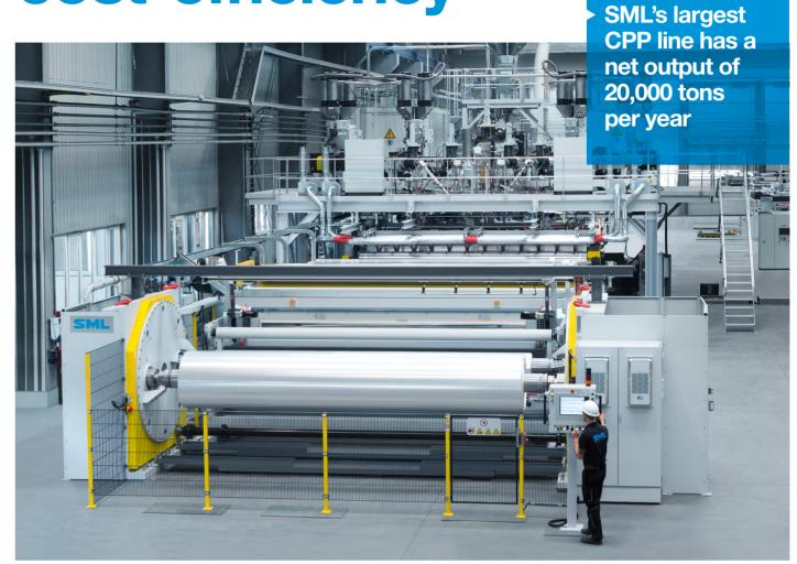
Extra-wide CPP film lines are a costefficient solution when it comes to the high-volume production of CPP film for metallisation. SML offers extrawide cast film lines for the production of CPP film for the packaging of food and textiles, especially for metallised CPP lamination films, which are highly popular in Asia. These CPP lines are typically 5-layer lines with film widths ranging up to 6.5m.
