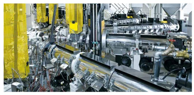
EXTRUDER ARRANGEMENT OF A BARRIER SHEET LINE A
