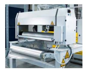
Inline thickness measuring unit with inductive/capative sensor
