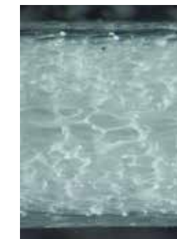
Cross section 3-layer sheet with foamed middle layer
