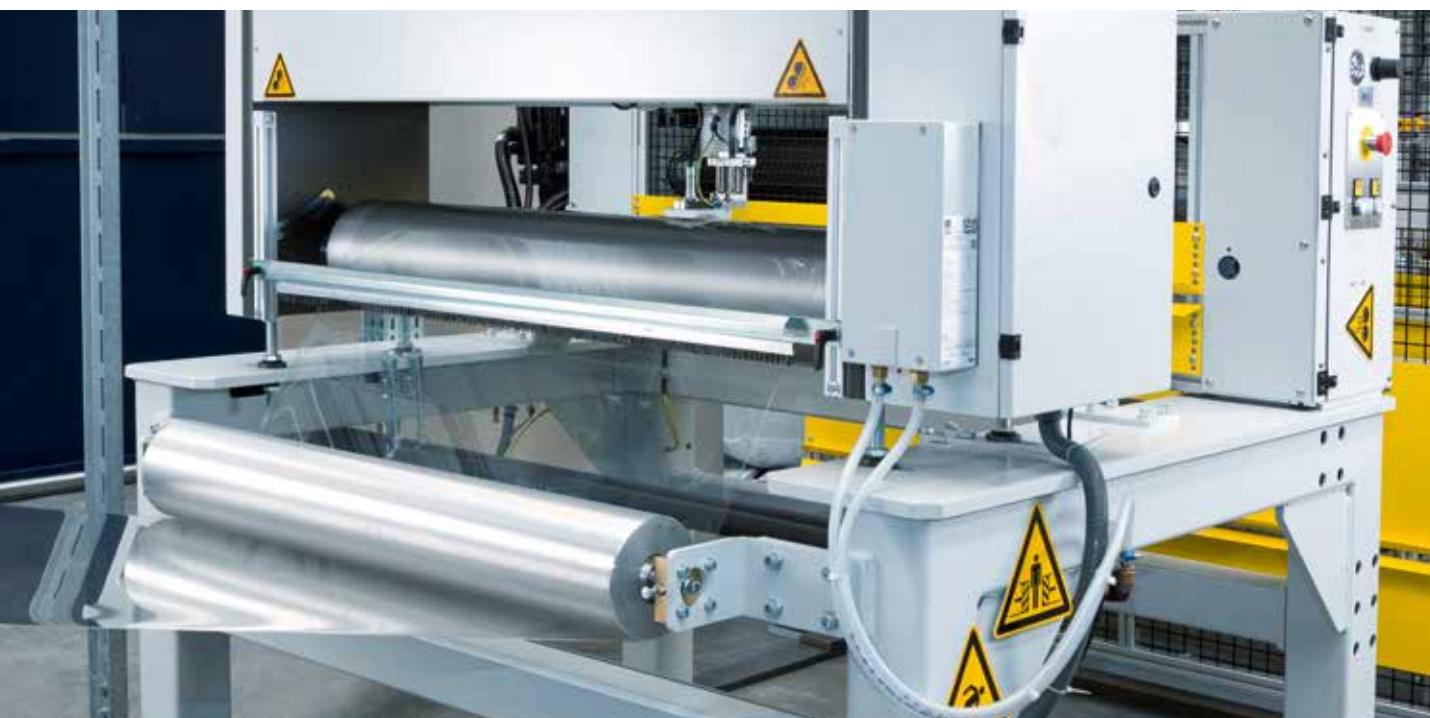
INLINE THICKNESS MEASURING UNIT WITH INDUCTIVE / CAPACITIVE SENSOR ▲
