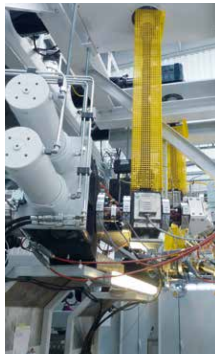
Tool unit with continuous double-piston filter and melt pump
