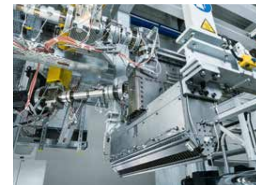
Tool unit with melt pump, static mixer, feedblock and flat die
