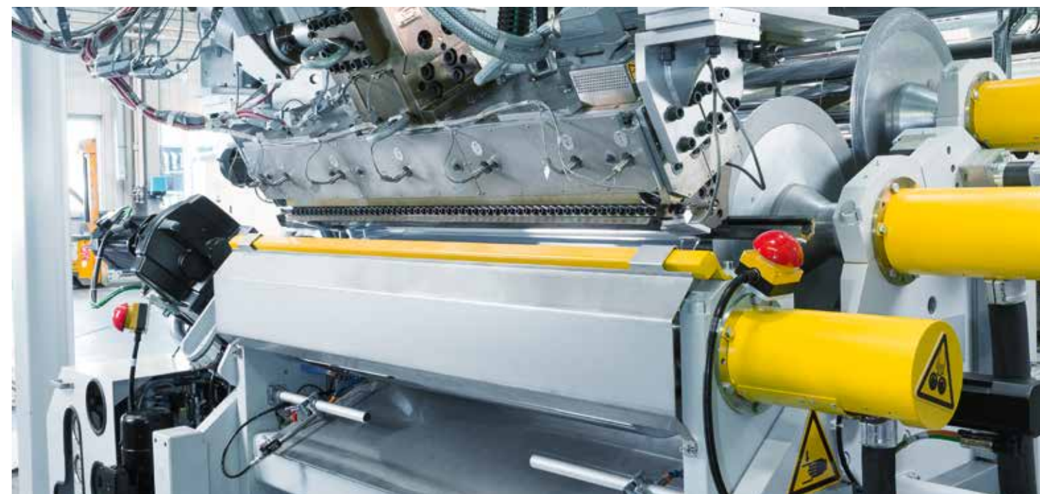
INCLINED ROLL STACK ▲
