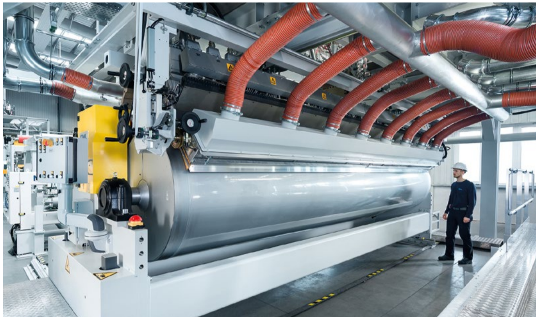
SML wide CPP film line at PT Panverta
