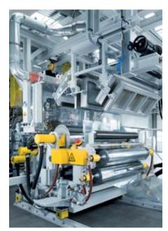
The second aspect of SML's approach to the PET issue involves down-gauging and physical foaming. The former may involve the use of a MDO orientation unit, which facilitates the production of films in a
