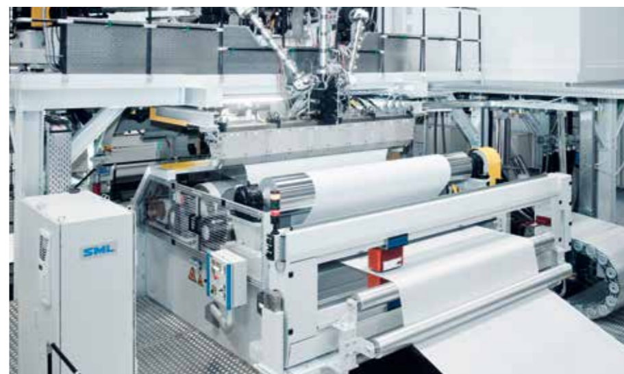
melt embossing unit with thickness measuring frame
