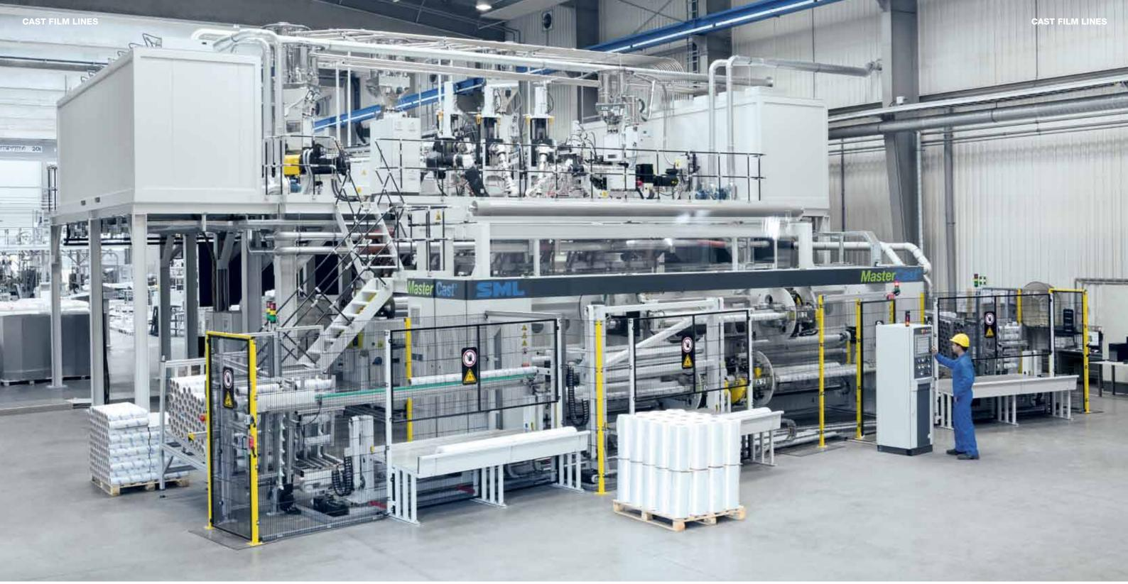
MasterCast\* Stretch Film Extrusion Line
