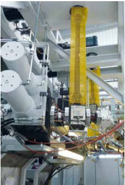
tool unit with continuous double piston filter and melt pump
