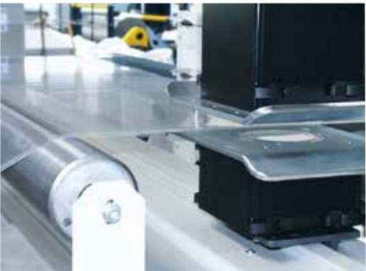
inline thickness measuring unit with Beta-ray sensor
