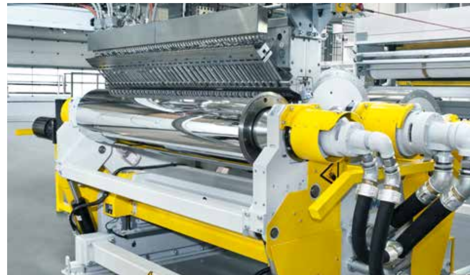
horizontal roll stack
