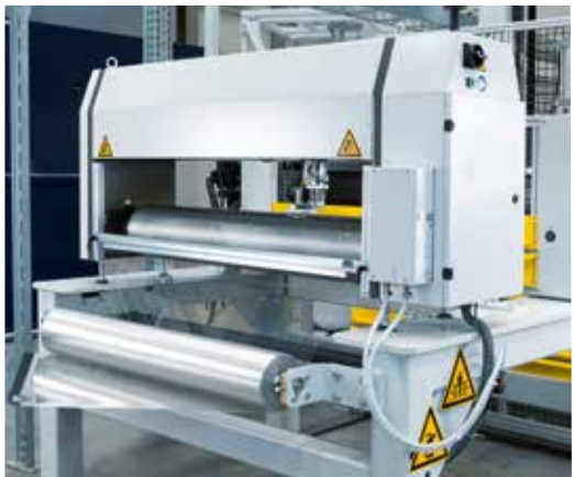
inline thickness measuring unit with inductive/capative sensor
