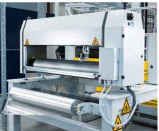
Inline thickness measuring unit with inductive/capacitive sensor
