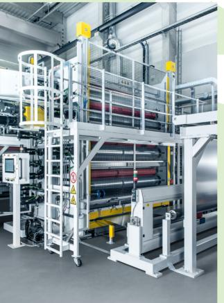
Demand for MOPE, MOPP and MOPET film has been rising sharply during the last two years. The main reasons for this phenomenon are the better recyclability and the lighter weight of the packaging materials. SML's further-developed MDO unit for cast film is the ideal technology for manufacturing these types of film.
