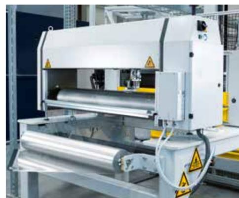
Inline thickness measuring unit with inductive/capative sensor
