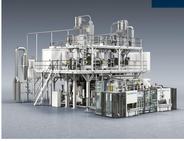
defined bin. The operator no longer needs to empty the dosing chamber manually. The seven extruders supply the stretch film material to a proven 13-layer feed block, connected to the latest Cloeren Reflex™ die. In combination with the X-ray gauging system, the SML Booster technology and the SML Automapping, manual adjustments on the die are no longer required.
