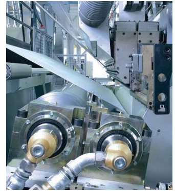
Laminator unit of a coating line for nonwovens
