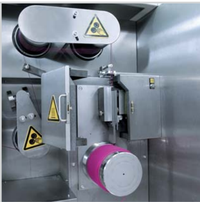
SML's patented texturing jet ▲
