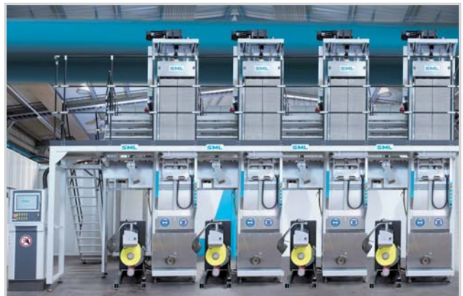
Austrofil POY line-by-line comprising 4 modules
