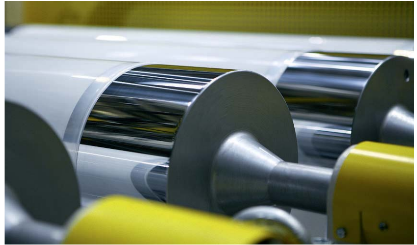
Post-cooling roller unit
