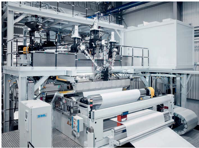
Production line for hygiene backsheet
