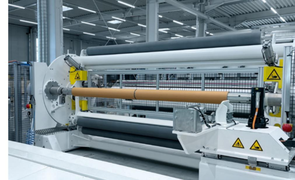
The coating of wide products has been one of the core competencies of SML for decades. One characteristic all these lines have in common is a **very massive machine frame** to withstand the high web tensions and **to avoid vibrations.**
