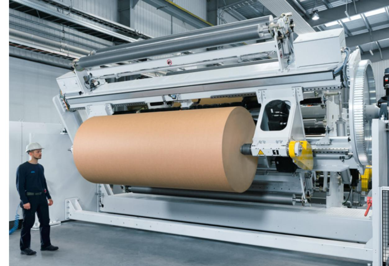
Splicing can be done up to full production speed. Core clamping is done shaftless by mechanically actuated chucking heads of various sizes.
